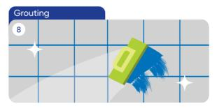
• Grouting should be carried out after 24 hours of tiling. It is advisable to use the appropriate grouting material from Magicrete range of cementitious or epoxy grouts.
