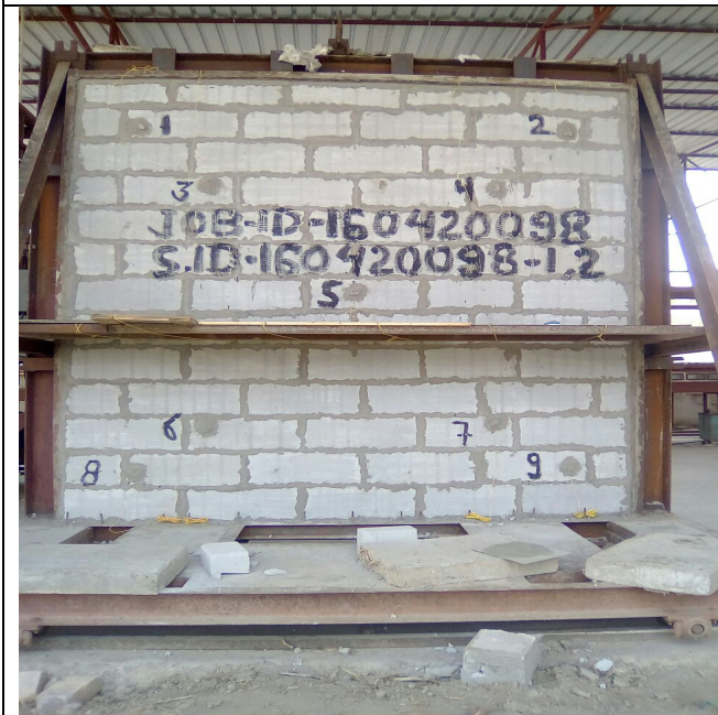
FIXING OF THERMOCOUPLE AT UNEXPOSED SURFACE
